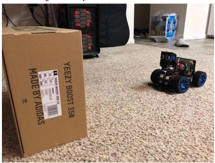
Finally, the ultrasonic sensor will be detecting the front of the Picar, and it will draw out a graph to shows the distance between the object and itself.
